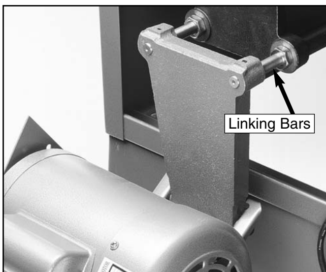
Figure 19. Attaching motor to linking bars.
